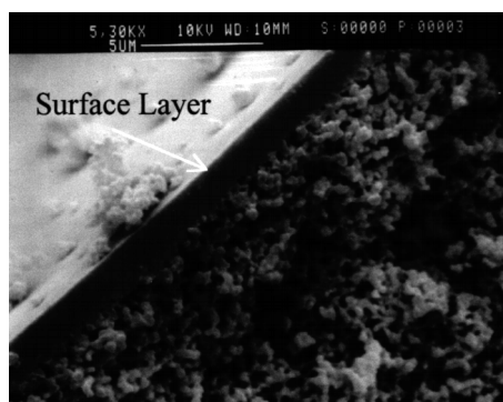
Figure 10. A sectional view of a 0.9-mm thick gel of f-DETA43W8-HCL38 gel showing a structurally compact surface layer.
